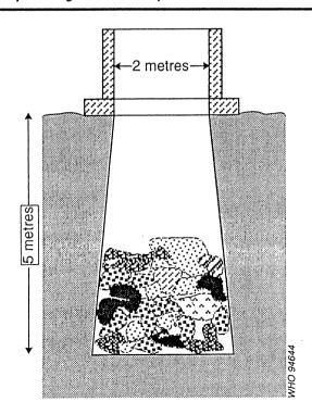
Protection from scavengers is best achieved by constructing a wall around the opening of the pit, which should not exceed 3 metres in diameter (see diagram).
