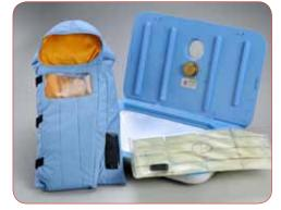
pouch is heated for 30 mins in the heater (second version uses boiling water instead of electrcity to heat) and then placed in the sleeping bag. It maintains the WHO recommended temperature of 37 deg C for 4-6 hours, after which it can be reheated.
