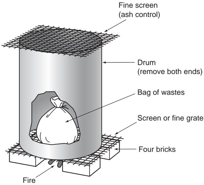
DMU incinerator for mixed
