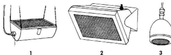
**Figure 11: Different types of safelights. Number 3 safelight is used over the dry bench, number 1 is the central indirect beam and number 2 is an optional safelight. The safelight in the centre of the ceiling should shine upwards, never downwards.**
