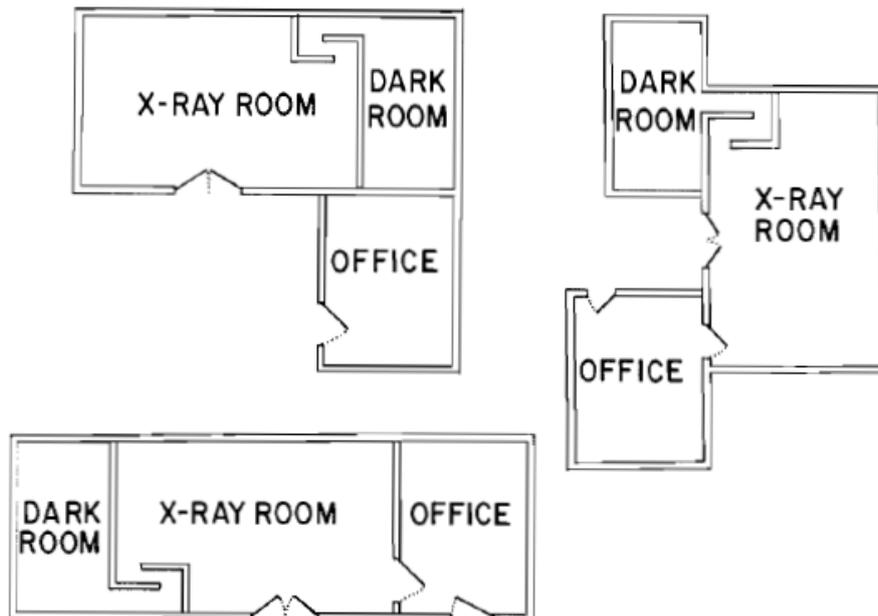
**Figure 1: Alternative room layouts for a radiographic suite**
